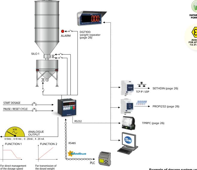
Example of dosage system using the **DGTQF** for loading routine
