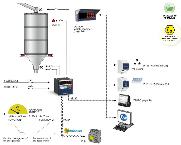
Example of dosage system for discharging with the DGTQF
