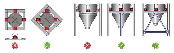
It is necessary to study with great attention the placement of the load cells and the mechanical features of the structure, avoiding any irregular
