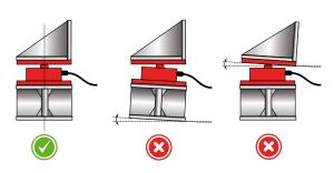
For a correct functioning of the weighing system and to obtain the best accuracy:
