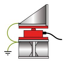
The grounding of the structure is indispensable to guarantee an optimum protection of the load cells from electrostatic discharge. A bridge between the upper plate and the lower plate of the kit is necessary and it could be created by using a cable or a copper braid of appropriate diameter.
