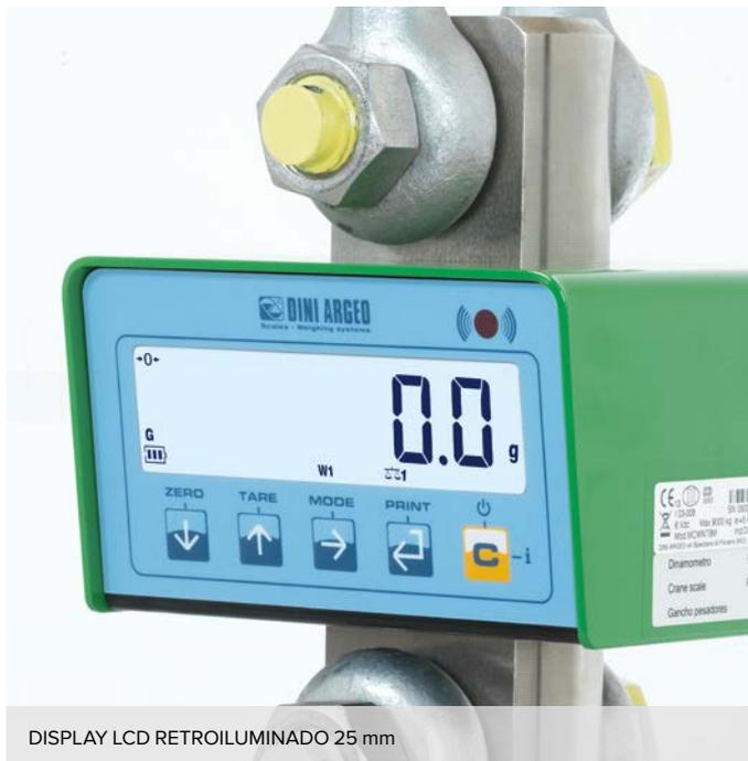
DISPLAY LCD RETROILUMINADO 25 mm
